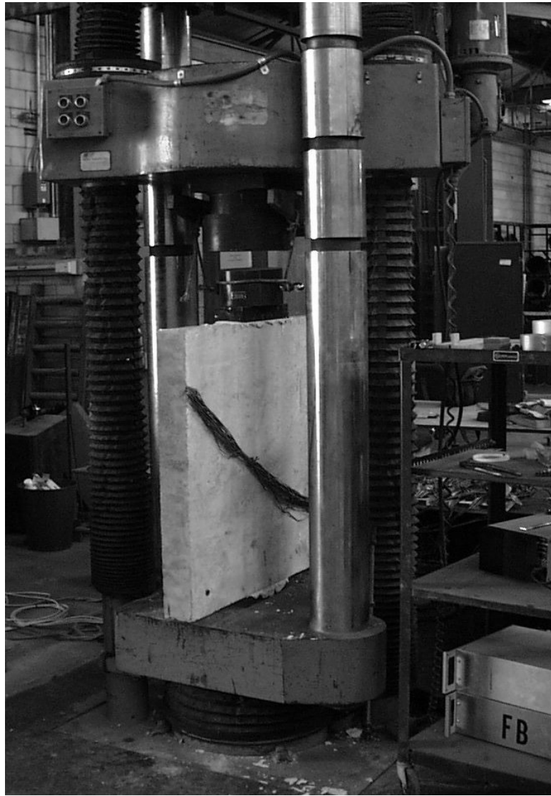
Figure 3-3: Testing of an isolated strut specimen
