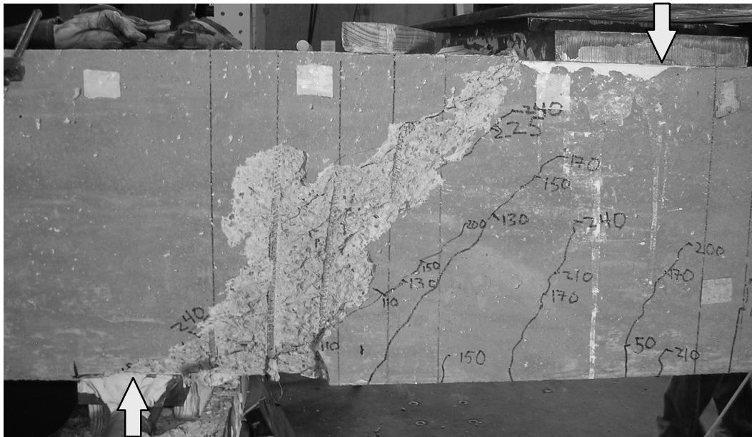
Figure 4-22: Typical failure of the North shear span in Series II specimens (Specimen II-N-F-5.8-3)
